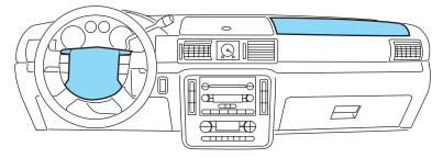
The airbag supplemental restraint system (SRS) is designed to work in conjunction with the safety belts to help protect the driver and front outboard passenger from certain upper body injuries. The term "supplemental restraint" means the airbags are intended as a supplement to the safety belts. Airbags alone cannot protect as well as airbags plus safety belts in impacts for which the airbags are designed to deploy, and airbags do not offer any protection in crashes for which they do not deploy.
